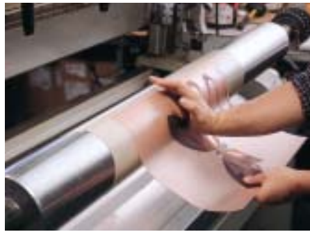
Apply plate to cylinder using the same method described above for the tape.
