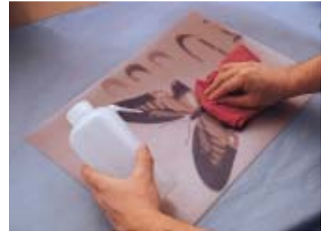
Insure that the back of the plate is clean prior to mounting.
