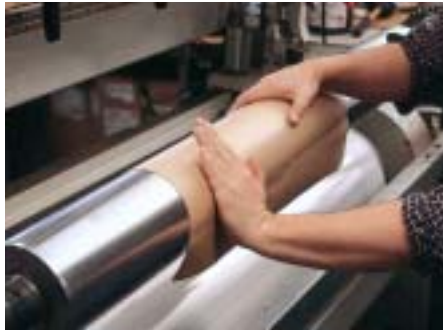
Apply tape to cylinder using light pressure with the palm of your hand or a squeegee. Avoid using fingertips as this will apply uneven pressure and increase likelihood of bubbles.
