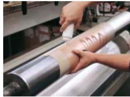
For long runs with aggressive plate-cleaning techniques use edge seal to insure trouble-free operation.
