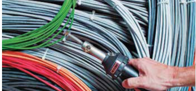
Fitting a solder shrink connection with the HOT JET S outfitted with a push-fit sieve reflector.
