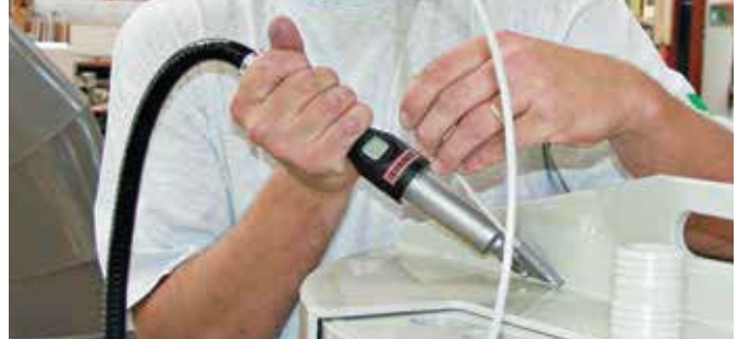
Draw welding using the compact and lightweight WELDING PEN R.
