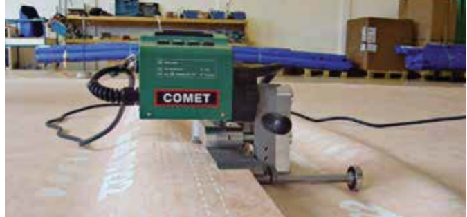
Hands-free welding due to integrated guiding plates.
