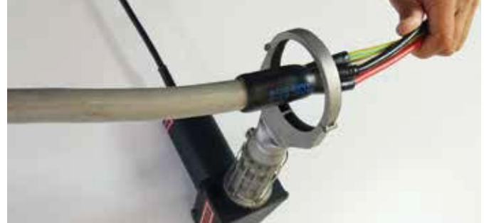
Shrinking cable connections which the GHIBLI.
