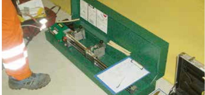
Seam tests can be conducted in the labor on-site with the EXAMO USB.
