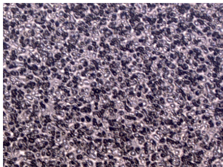
Cyrel® Performance Plate engineered surface (@ 200 magnification)
